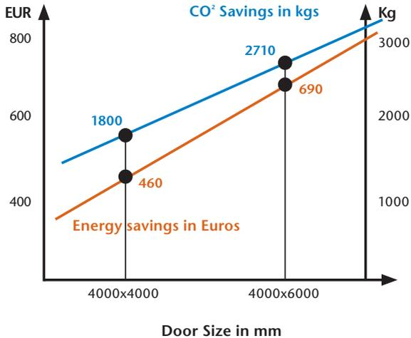
Assumptions: 1) Cold air flow assumed by 5°C outside temperature and 20°C interior temperature metered in m<sup>3</sup>/h related to m<sup>2</sup> gate opening (existing from building geometry and wind load). 2) Thermal efficiency factor for heat supply: 85% 3) Price of fuel oil: 0,77 EUR/l (based on: 01.02.2011)
